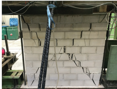
Figure 13. CS_S1: calcium-silicate brick masonry wall strengthened on one side. Cracking pattern and equivalent multilinear curve.
